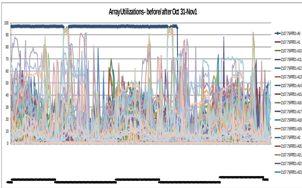
The problem was in a performance monitor inappropriately dumping to logs on array 0.
