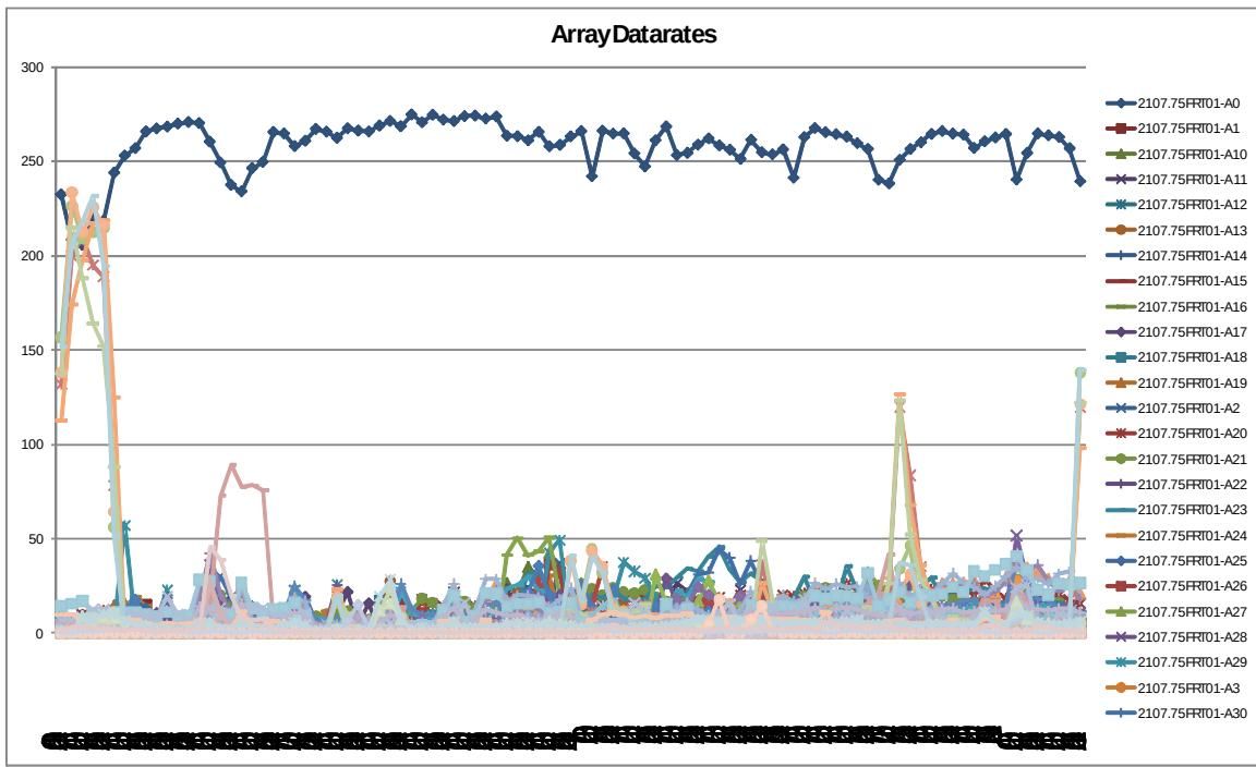
Array 0 is swamped !! The load impacts all the applications that depend on the array.
